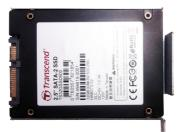
Assemble the storage device to the storage bracket.
