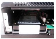
Fully slide the storage bracket and the storage device until they cannot be slid any more.
