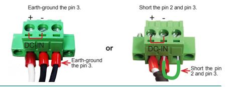
7. Use a slotted screwdriver to tighten the captive screws. Plug the terminal block firmly, which wired, into the power receptacle at the bottom of the computer.
