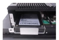
Slide the storage and the bracket back into the computer.
