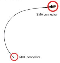
8. Connect the RF antenna's MHF connector to the Wi-Fi module's "MAIN" connector.
