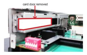
4. Plug a PCI (or PCIe) card to the PCI (or PCIe) slot. Fully plug the card.
