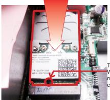
The notch on the Wi-Fi module should meet the break on the connector.
