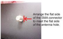
11. Mount the washer first and then the nut to the SMA connector. Make sure the nut is tightened.
