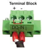
6. Either earth-ground the pin 3 on the terminal block or short the pin 2 and pin 3 on the terminal block.
