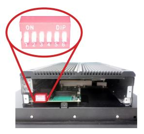
2. Find the DIP switch as the illustration above shows. Adjust the DIP switch to the desired data transmission protocol as described in 3.2.2. <u>DIP Switch</u> on page 23 for the serial port 1 (COM1) or the serial port 2 (COM2).
