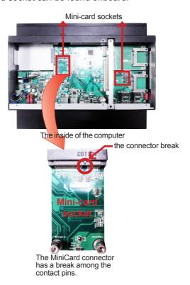
2. Prepare the **WIFI-IN1300** Wi-Fi module kit. The module is a half-size module of **PCI Express Mini-card** form factor, with two U.FL connectors, one is "MAIN", and the other is "AUX".
