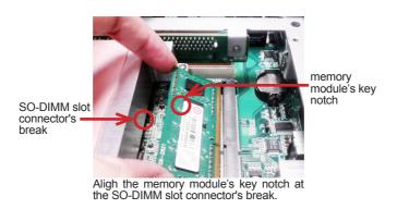
4. Fully plug the memory module until it cannot be plugged any more.
