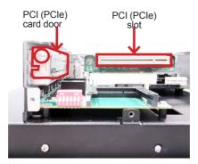
3. Remove the screw that fixes the card door as the illustration in **step 2** shows, and remove the card door.
