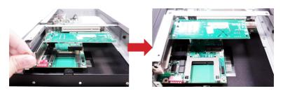
5. Refasten the screw to fix the card door.
