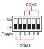
By default, all toggles are slid to **off** positions, which means both COM1 and COM2 are set to RS232 in default state. See the following guide for more details.
