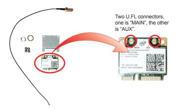
3. In order to make the half-size Wi-Fi module compatible with the **Mini-card** socket, extend the WiFi module with a "mini half bracket". Join them together by using two screws.
